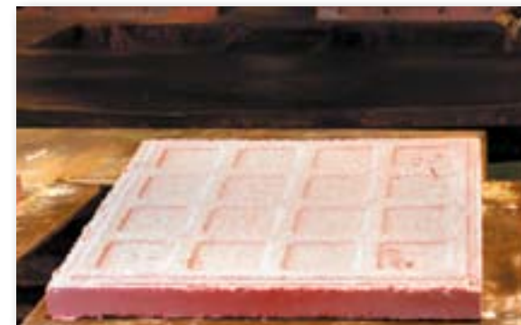
3. Sformatura/Remove tile from mould
