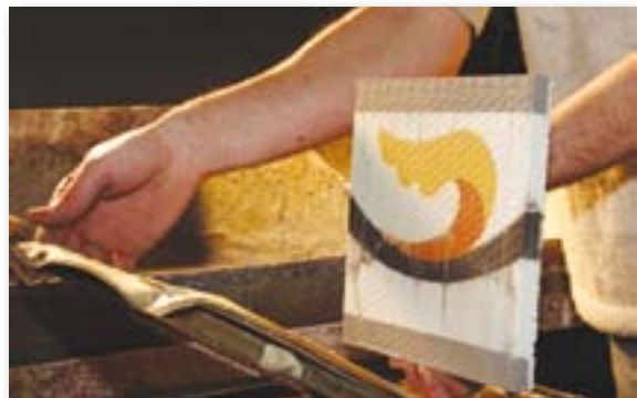
5. Sformatura/Remove from mould
